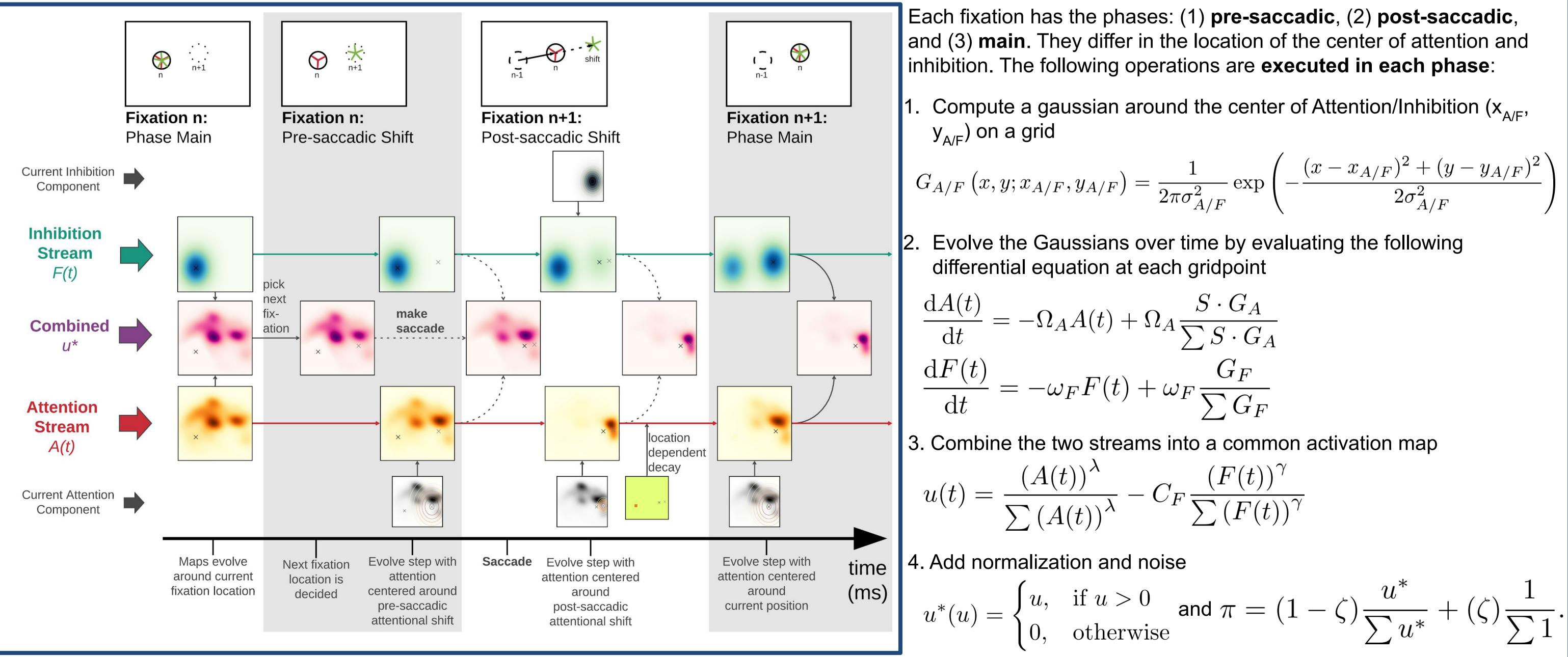
$$G_{A/F}\left(x, y; x_{A/F}, y_{A/F}\right) = \frac{1}{2\pi\sigma_{A/F}^2} \exp\left(-\frac{(x - x_{A/F})^2 + (y - y_{A/F})^2}{2\sigma_{A/F}^2}\right)$$
